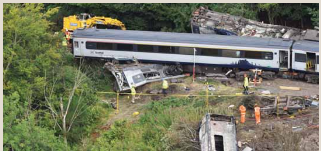
DISASTER: The Rail Accident Investigation Branch report into the disaster at Stonehaven, Carmont, where three people lost their lives, found that the failure to ensure inspections were carried out on a drainage system directly contributed to railway engineers not identifying a construction fault which ultimately led to the derailment.
