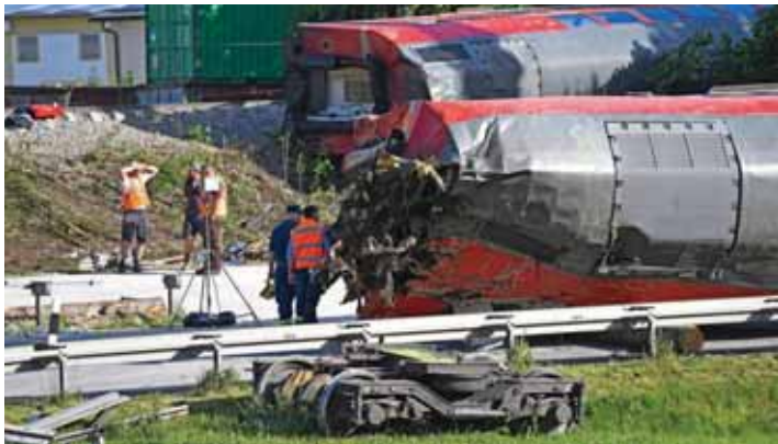
DERAILED: Derailed DB train due to a switch failure, Berlin Tegel on August 21, 2012
