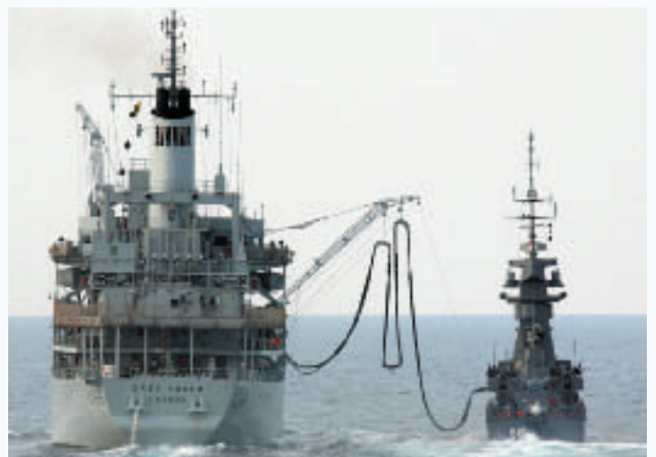
REFUELING: RFA Grey Rover refuelling Singapore Navy corvette Victory off the Malaysian island of Palau Tioman.
